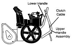
Reference to the right or left hand side of the snow thrower is from the operator's position behind the unit.
